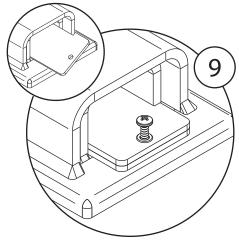
(Slide in adaptor plates diagonally if required.) Add washers and M6 bolts (longer bolts with more adaptor plates) to complete the installation.
