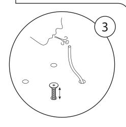
Use the hose to blow out all dust inside the hole. A bolt can also help to scrape dust away.
