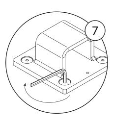
Using the Allen Key (or Hex Drive bit with a 1/4" socket), tighten all the bolts.
