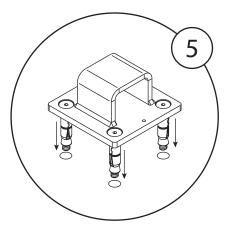
Align and push the baseplate so the bolts and shield anchors go into the drilled holes.
