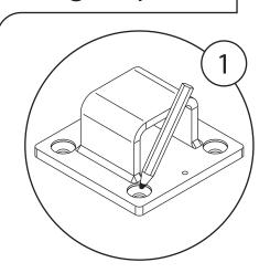
Place the baseplate at the desired location and mark the holes to drill.
