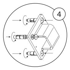
Away from the wall, push all bolts through base plate and **loosely** attach shield anchors.
