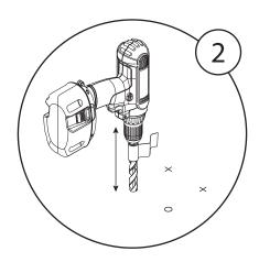
Drill each hole perpendicular to the wall until the tape touches the surface (at 70mm depth).
