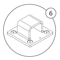
Ensure that the baseplate and bolts are firmly against the mounting surface.
